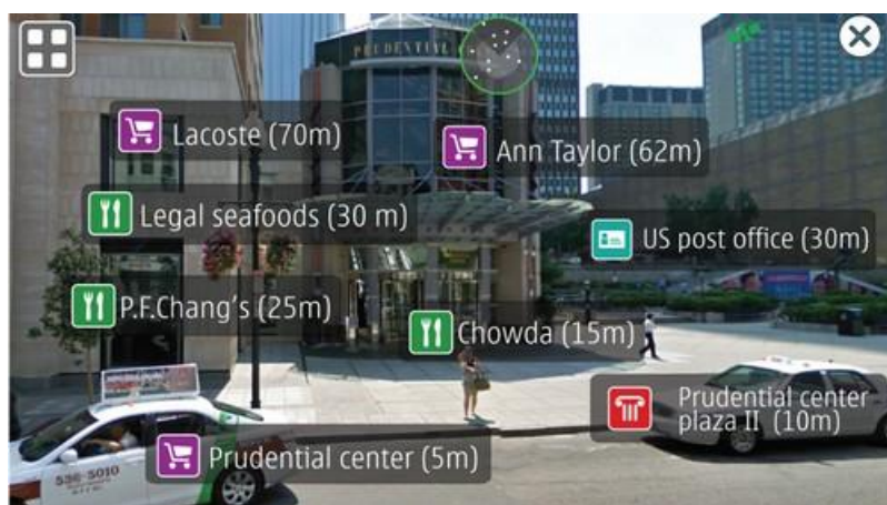
Figure 4.2.1: Augmented reality refers to the insertion of virtual elements into a real video scene. As an example, the figure shows a screenshot of a smartphone application by Nokia Beta Labs called LineView, which was recently announced (July 2011). This augmented reality browser, with the use of GPS and camera, displays real time information about the points of interest around your location.
