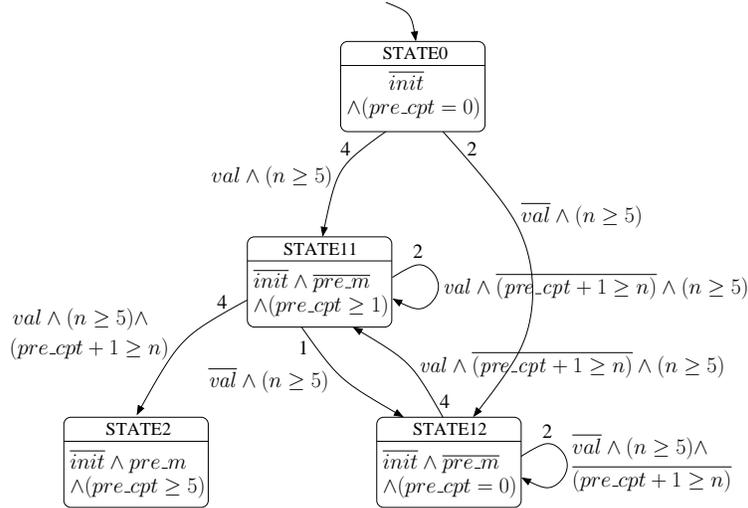
**Fig. 7.** The Lucky automaton: adding weights to the result of Nbac shown on Figure 5
