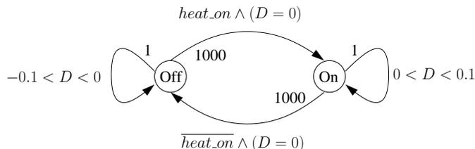
**Fig. 6.** A simple Lucky automaton with a Boolean input *heat\_on* and a float output *D*
