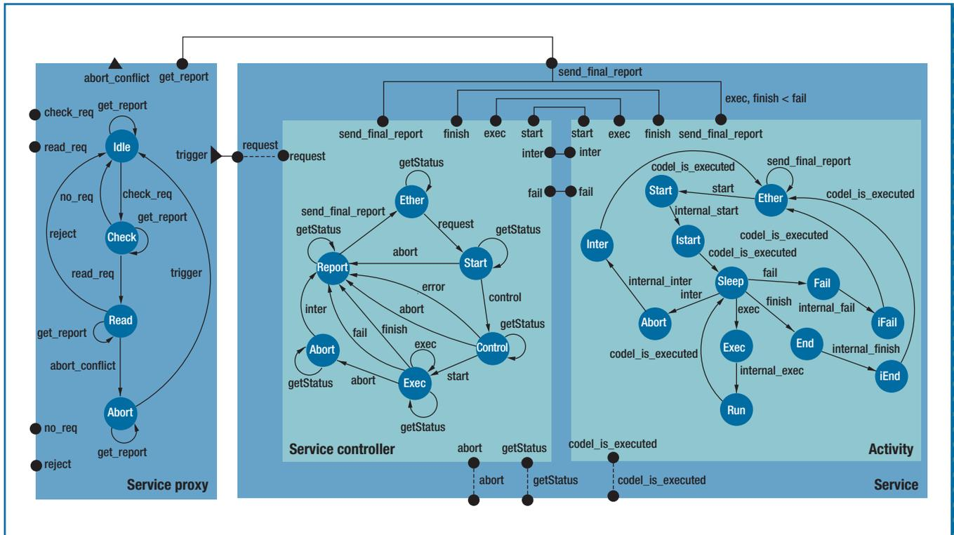
**FIGURE 1.** BIP component schematic. The **Service** composite component on the left, for a Dala robot service, consists of two atomic components: **Service Controller** and **Activity**.
