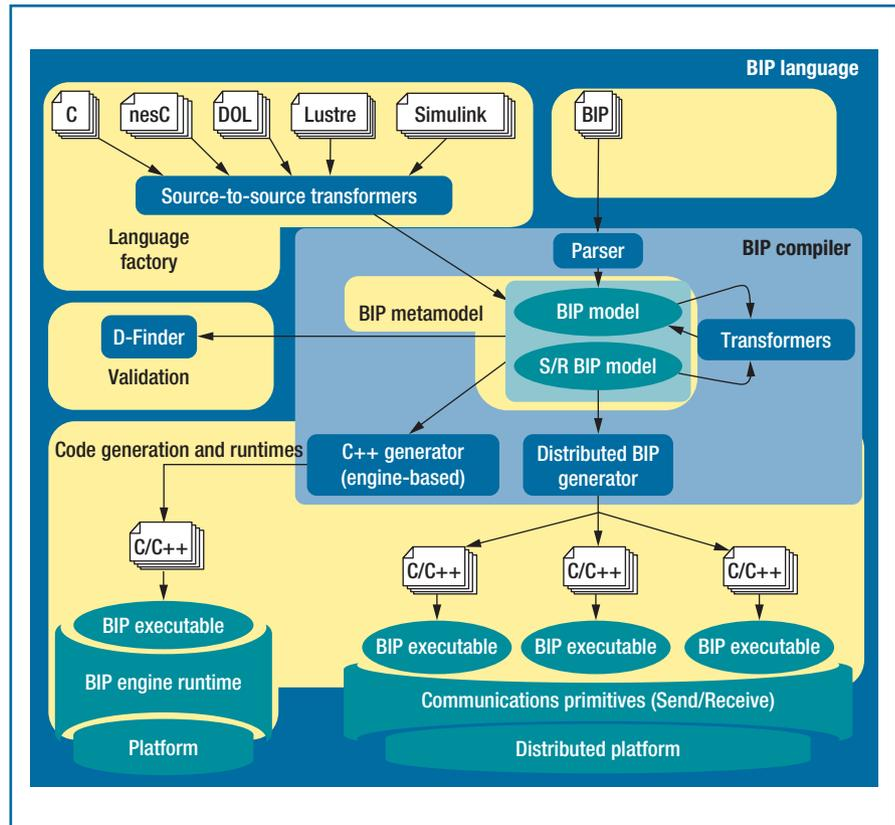
**FIGURE 3.** BIP toolset. The tools include translators from various programming models, verification tools, source-to-source transformers, and C/C++ code generators for BIP models.
