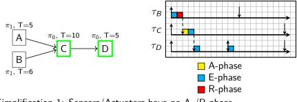
Simplification 1: Sensors/Actuators have no A-/R-phase Simplification 2: E-phases handle **colocated** communications Simplification 3: Remove redundant data-dependencies
