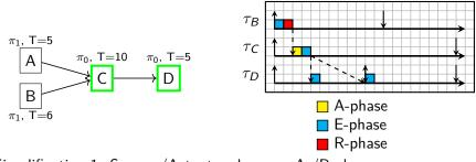
Simplification 1: Sensors/Actuators have no A-/R-phase Simplification 2: E-phases handle **colocated** communications
