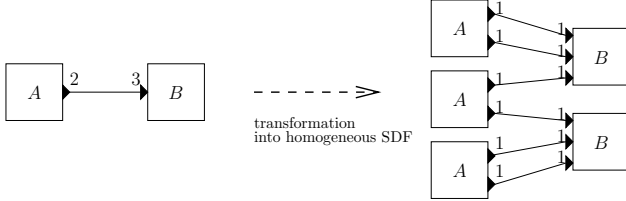
Figure 2. Example of SDF diagram and transformation into homogeneous SDF proposed by Lee and Messerschmitt.
