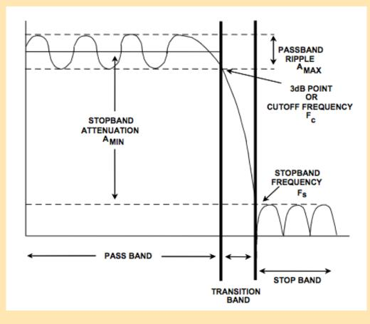
The stop band frequency is generally  $\frac{1}{2}$  the sample rate, i.e.  $\frac{1}{2T_e}$
