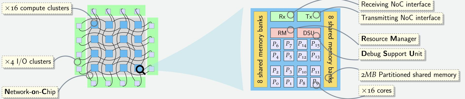
Massively parallel processor with low power consumption and a predictable design
