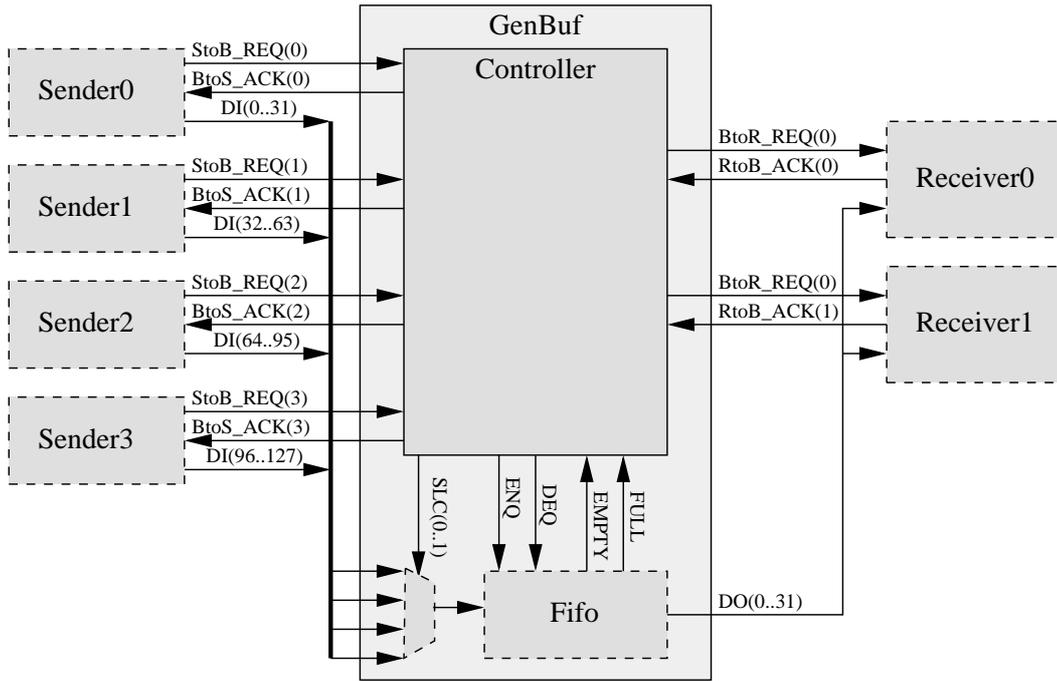
Fig. 4. Block diagram of GenBuf with four senders
