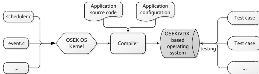
**Fig. 1.** Traditional approach to implementing an OSEK/VDX-based operating system
