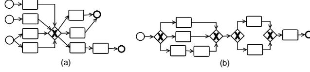
**Fig. 2.** (a)well-structured BPMN model. (b)well-formed BPMN Model.
