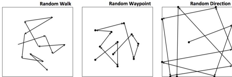
**Fig. 1.** Motion paths of a mobile node in three mobility models, where a bullet  $\bullet$  depicts a pause in the movement.
