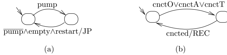
Figure 4.12: The pointcut (a) and the recovery program (b) for the recovery aspect.
