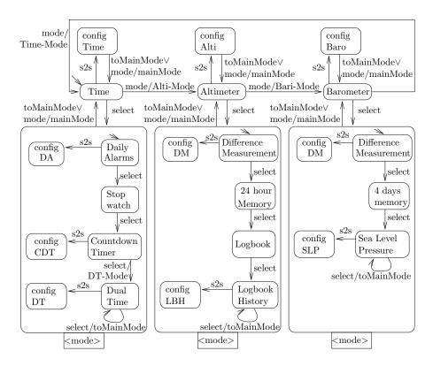
Fig. 7. The base-program component. Its interface is: inputs = {Mode, Select, plus, minus, s2s}, outputs = {Time-Mode, Bari-Mode, Alti-Mode, mainMode}, toMain-Mode is encapsulated.
