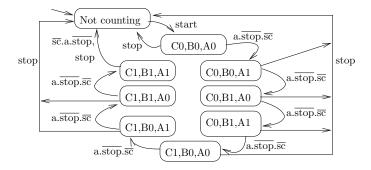
Fig. 2. The behavior of the modulo-8 a-counter
