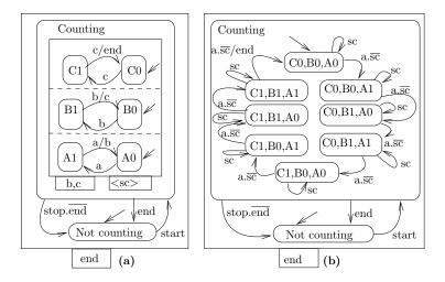
Fig. 1. Two Argos programs for the modulo-8 a-counter
