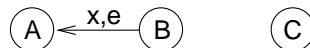
Figure 9: Static Dependency Graph for the foobar example. Nodes represent processes. Arrows represent possible communications between processes. An arrow goes from the master (i.e. the notifier for a SystemC event, the writer for a shared variable) to the slave.
