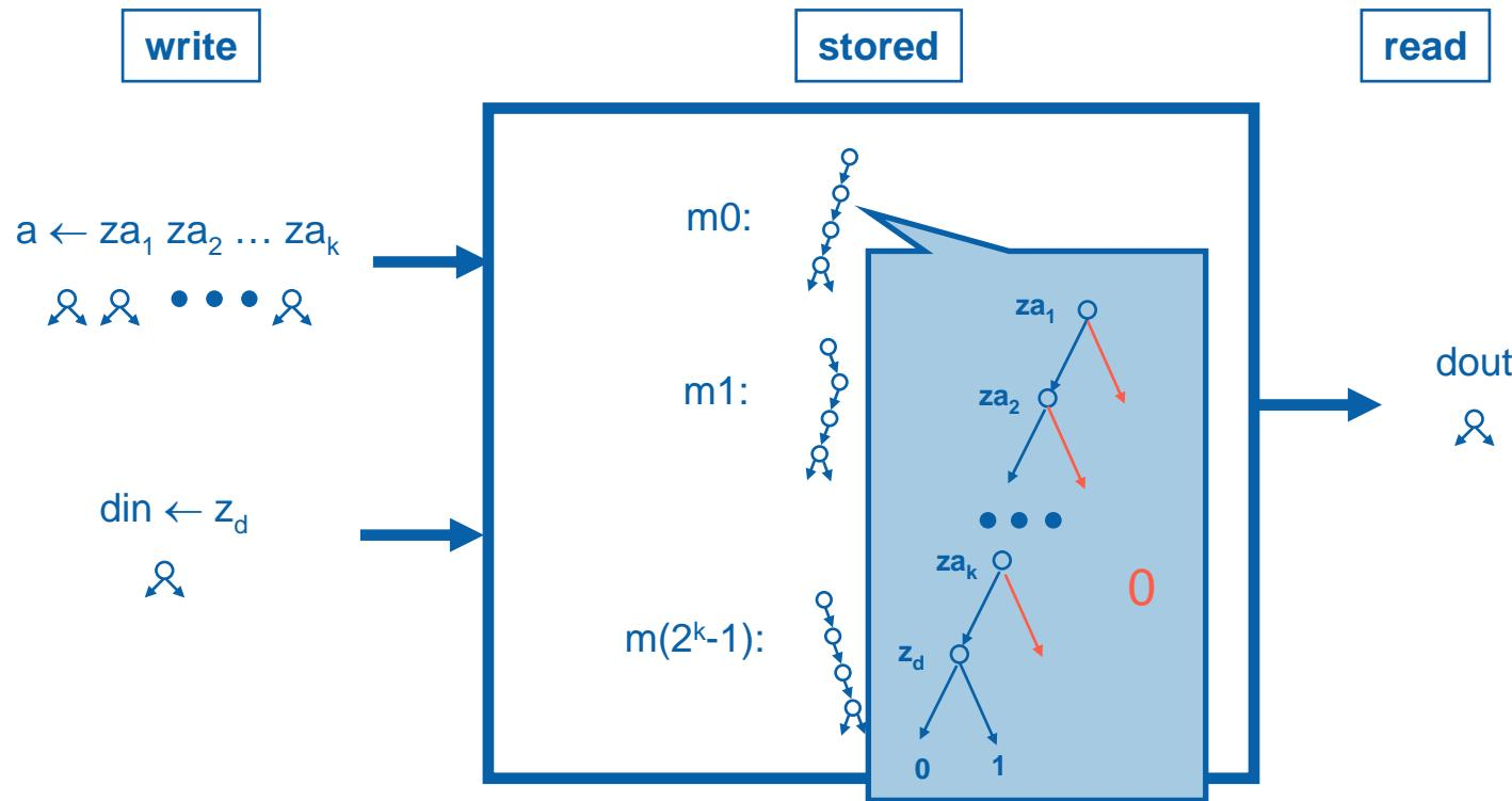
For an  $n=2^k$  cell memory, the size of all the BDD nodes in a single rail is:
