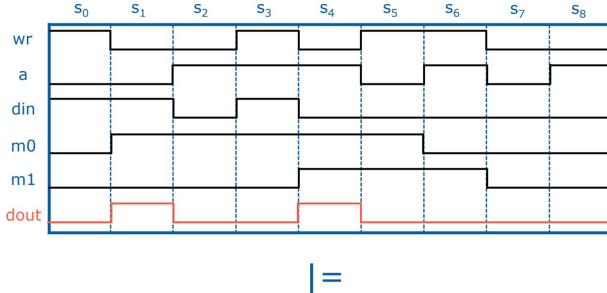
$(wr \& a=z_a \& din=z_d, 1) \quad (!wr \& a=z_a, dout=z_d)$
