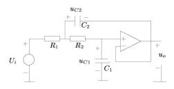
Fig. 2. A low-pass filter.
