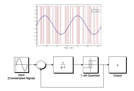
Fig. 4. A first order  $\Delta$ - $\Sigma$  modulator and an example of an input-output plot.
