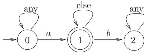
Figure 1.7: A Büchi-automaton monitor for checking an unbounded-response property.
