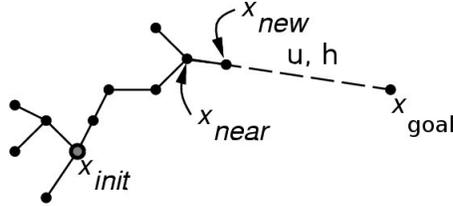
Figure 1.16: Illustration of one iteration of the RRT algorithm.
