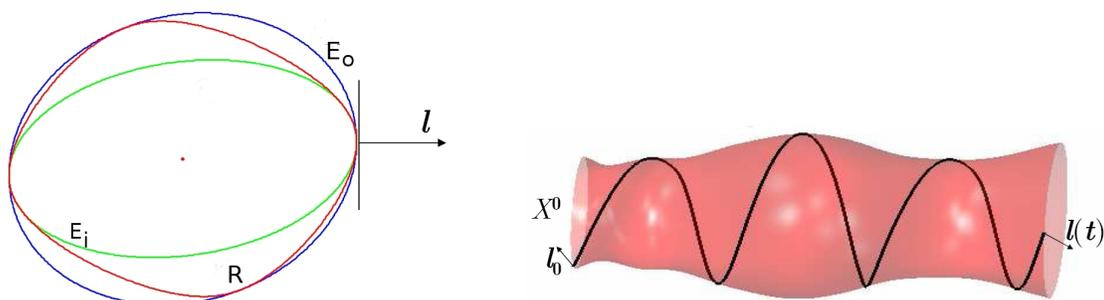
Figure 1.10: Reachability computation using ellipsoids [68].
