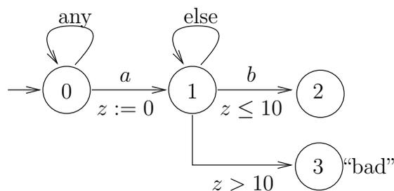
Figure 1.5: A timed-automaton monitor for checking a bounded-response property.
