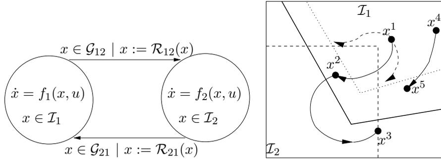
Figure 1.4: A hybrid automaton and its trajectories.
