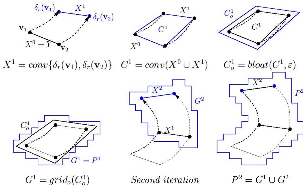
Figure 1.8: Illustration of the reachability technique for linear systems using convex polyhedra.
