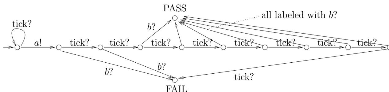
Figure 1.23: A digital clock test generated from the specification  $S$  shown in Figure 1.18 and the left-most, perfectly periodic, Tick model shown in Figure 1.21.
