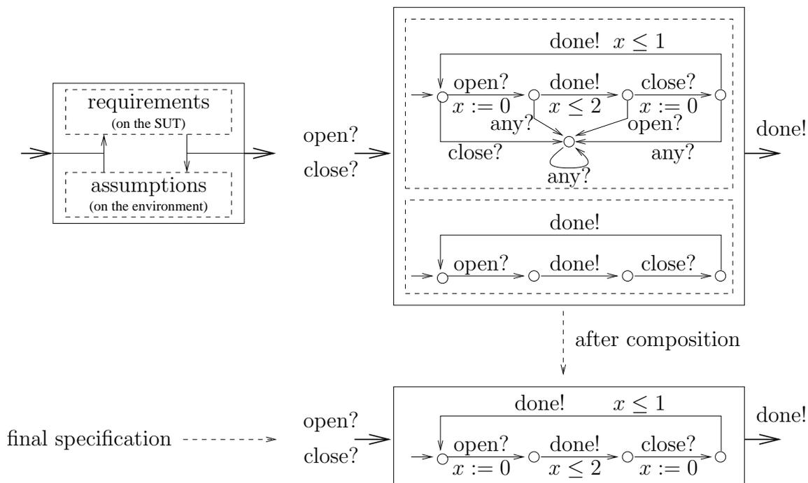
Figure 1.19: Specification including assumptions on the environment: generic scheme (left) and example (right).
