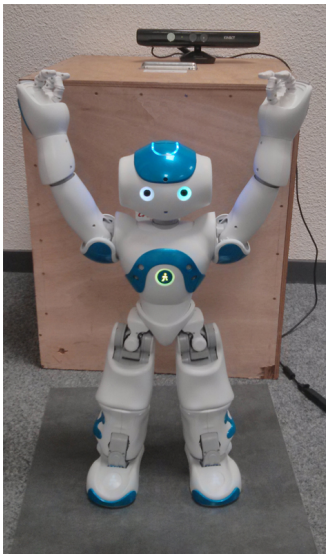
Figure 1: Setup for the imitation game. The RGB-D sensor overhangs the NAO and tracked the gamer skeleton.
